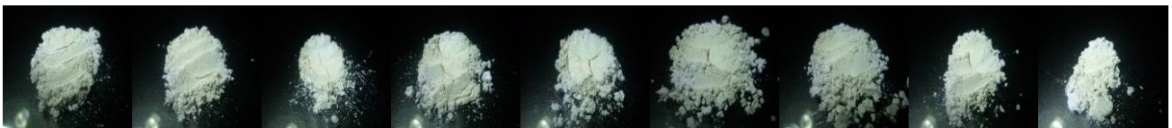
Silver Pearl Irradiant White Rutile Silver Silk Silver Bright Pearl Fine Satin White Silver Satin Luster Satin Flash White 10-60µm 10-70µm 10-60µm 10-40µm 10-50µm <15µm 5-20µm 5-25µm 10-100µm
