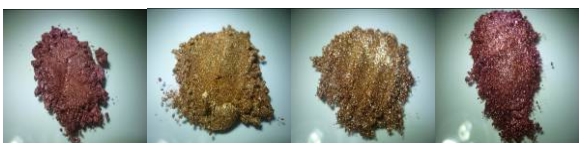
Satin Wine Red 5-25µm Bronze 10-60µm Flash Bronze 10-100µm Flash Wine Red 10-100µm
