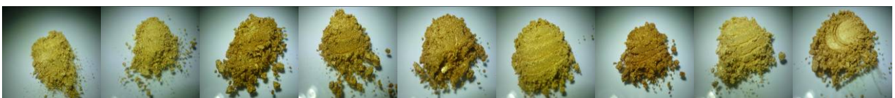
Gold Pearl Gold Satin Royal Gold Maya Gold Aztec Gold Olympic Gold Abtruse Gold Turquoise Gold Fine Satin Gold 10-60µm 5-25µm 10-60µm 10-60µm 10-60µm 10-60µm 10-60µm 10-60µm <15µm
