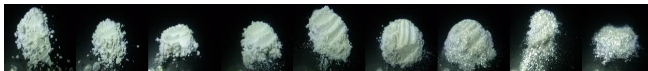
Fine Satin White <15µm Satin White 5-25µm Bright White 10-60µm Luster White 15-75µm Flash White 10-100µm Glitter White 30-150µm Sparkle White 40-300µm Ultra Sparkle White 50-350µm Intense Sparkle White 200-700µm
