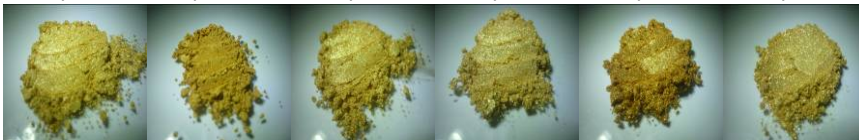
Bright Gold Satin Royal Gold Flash Gold Flash Red Gold Glitter Gold Shimmer Gold 10-60µm 5-25µm 10-100µm 10-100µm 20-120µm 20-200µm
